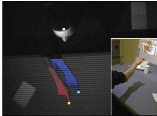
Fig. 14. Encumbrance-free interaction using imperceptible structured light (inset illustrates what the user sees).
