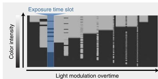
Fig. 13. Light modulation of a DLP projector.
