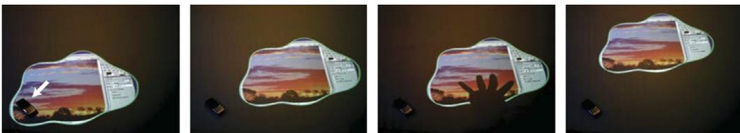
Fig. 16. Environment-aware display adaptivity based on imperceptible structured light scanning enabled by synchronized projection and capture. The display reacts to the colliding cell phone and subsequently avoids the shadow cast by the hand by dynamically relocating to an adequate area determined by the scanning of the projection surface.
