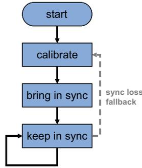
Fig. 5. SGL application control flow.
