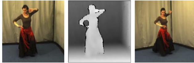
Fig. 9. Our 3D video system acquires color images of moving scenes (left) with corresponding depth maps (middle) which are used for re-rendering the video from novel views (right).
