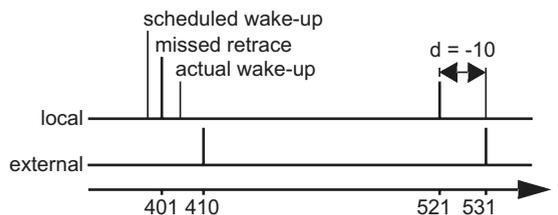
Fig. 6. Deviation ( $d$ ) between the local video timing and the external reference signal.
