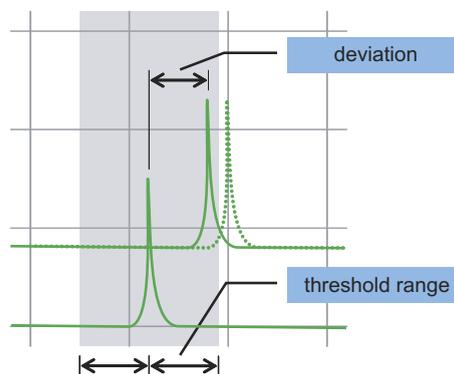
Fig. 7. Threshold for deviation.
