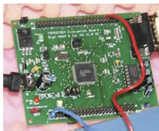
Fig. 4. Microcontroller for generating clock signal.
