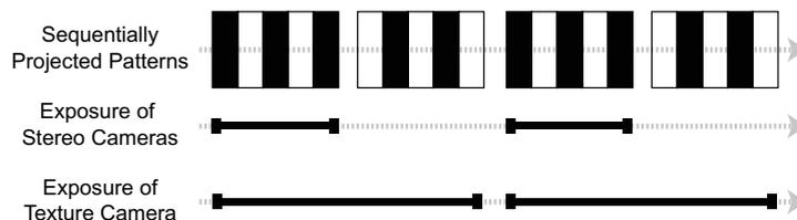
Fig. 11. Camera exposure with inverse pattern projection.
