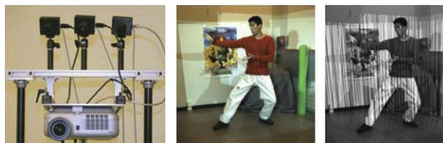
Fig. 10. 3D video brick with cameras and projector (left), simultaneously acquiring textures (middle) and structured light patterns (right).
