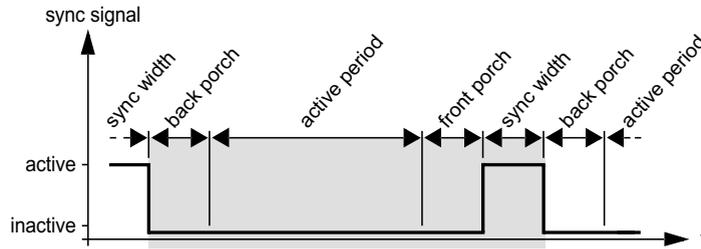
Fig. 2. Sequence of timing components.
